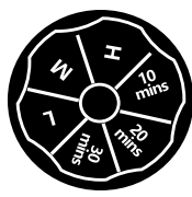
Sensitivity Dial calibrate spray time
